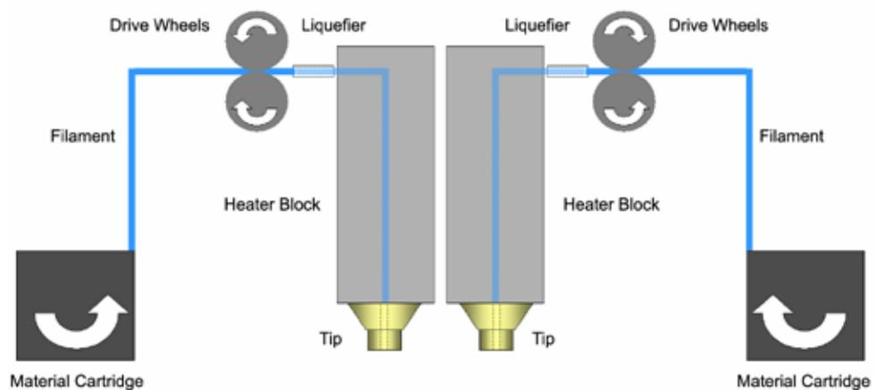
The FDM process with dual-tip technology.
